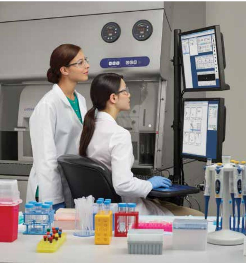
The BD FACSAria Fusion uses BD FACSDiva software to efficiently control the setup, acquisition, and analysis of flow cytometry data from the operator workstation. Software control of key operations minimizes direct interaction with the sorter for an added level of biosafety protection.
