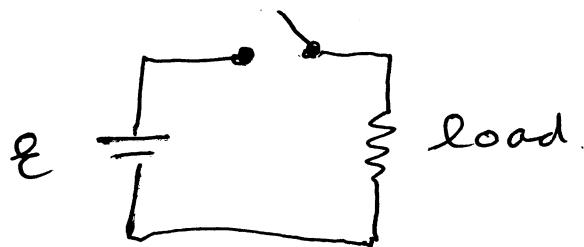
When switch is closed, current increases from zero and a magnetic field is set up:
