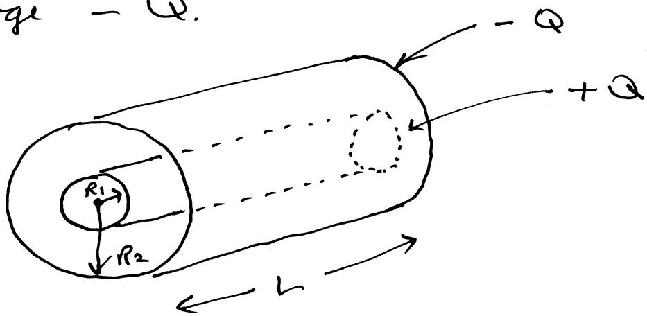
Due to the symmetry of the charge distribution, any electric field will be radial (inwards or outwards). Due to the symmetry of the charge distribution, any electric field is radial (pointing inwards or outwards) and has a
