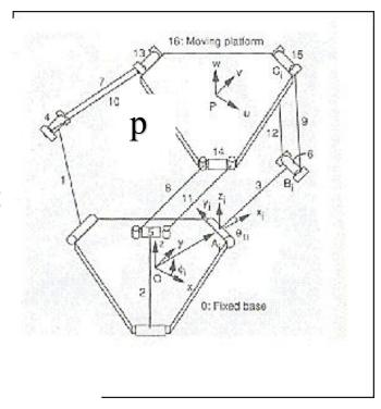
Given p we determine the location of point  $C_i$ . This is simple because the moving platform cannot rotate and thus the line between P and  $C_i$  translates only. Thus, given P (as determined by p) and the distance h, we can determine  $C_i$  as displaced from P by a vector of length h that is parallel to  $x_i$ .
