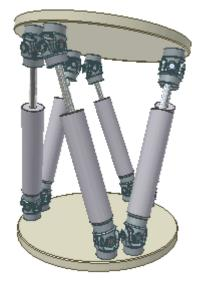
Spherical constraint:  $(\boldsymbol{p}_i - \boldsymbol{b}_i)^\top (\boldsymbol{p}_i - \boldsymbol{b}_i) = l_i^2, \ i = 1, 2, 3.$
