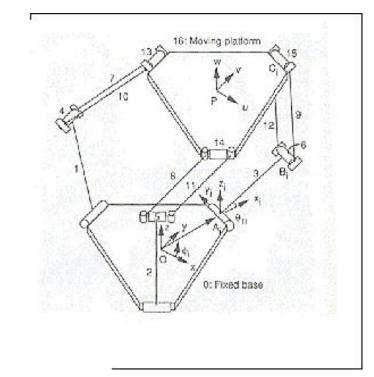
Assume that a desired position vector p given. Find the joint angles to place point P at p.
