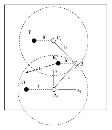
Given  $\theta_{3i}$  we can determine an equation for  $\theta_{2i}$  by summing the squares of the matrix equation to get
